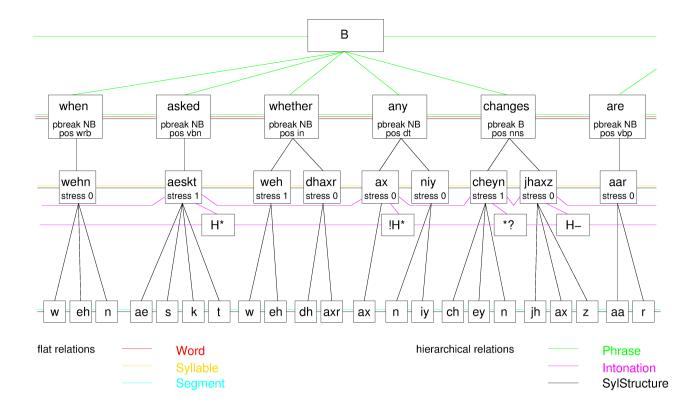
Some central linguistic or phonetic properties of the items are stored directly in the utterance structure in the form of features, such as part-of-speech, position of phrase breaks, and stress in the figure above. One of the most important properties, and **not shown** in the figure above, is the end time - it is stored as a feature for every single item. In our case, all these will have to be derived from the natural utterances, or more concretely, from label files for natural utterances.
